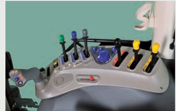
Cab with Efficient version: the controls of the P6-Drive transmission are integrated into the right-hand console.
